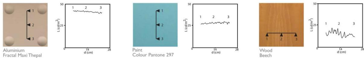
Figure 5: Photographs and measured luminance profiles for three samples lit by fluorescent lights.
