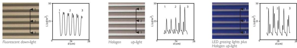
Figure 4: Photographs and measured luminance profiles for the corrugated aluminium sample under three different light conditions.
