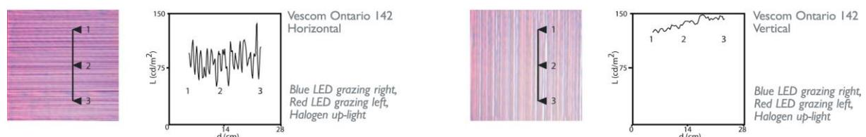
Figure 6: Photographs and measured luminance profiles for the differently oriented material samples.
