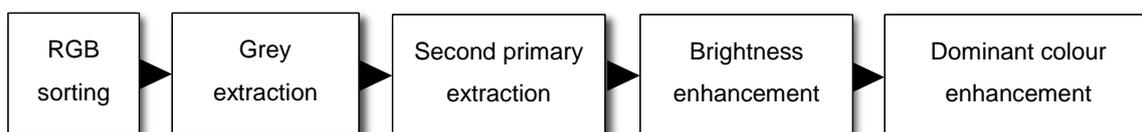
Figure 3: Colours separation flowchart.
