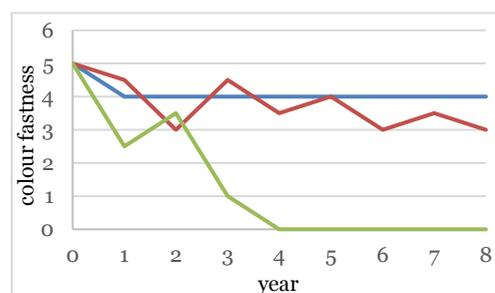
Figure 8: Colour fastness on white PVC windows in different environments. The colour fastness is represented according to the grey scale (CG) of DIN 54001 [15 p32].
