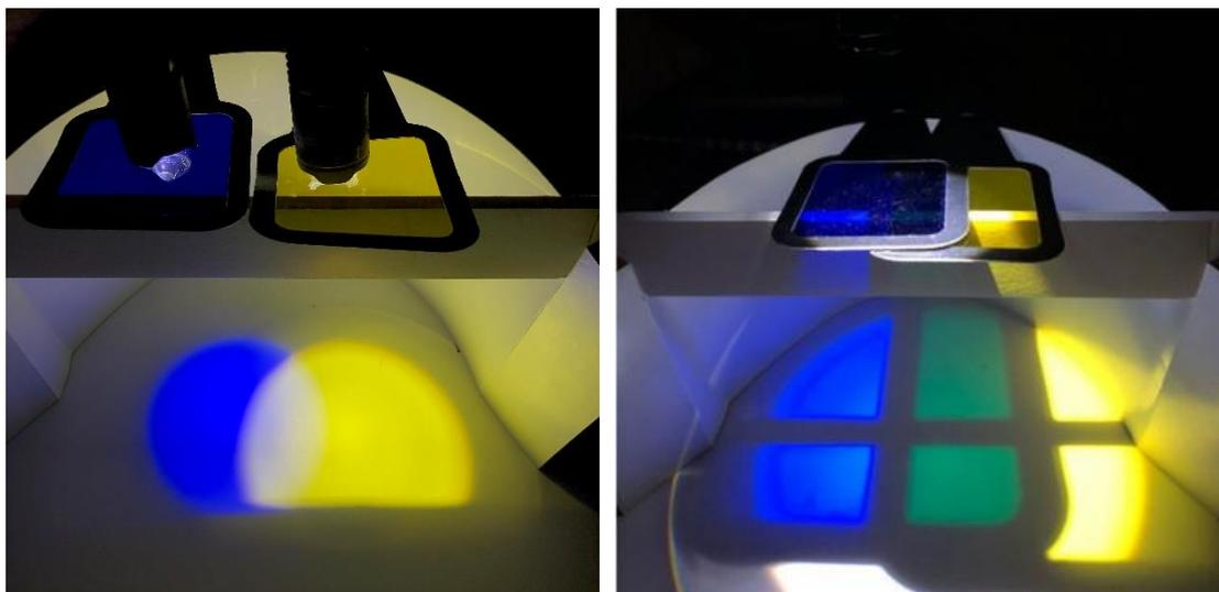
Figure 10: Combining separate blue and yellow- coloured light sources demonstrates the additive mixing process (left). Shining a single light source through stacked blue and yellow- coloured filters demonstrates the subtractive mixing process (right). Images courtesy of M. Maggio.
