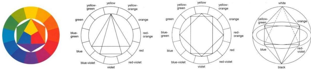
Figure 11: Johannes Itten's colour wheel with harmonies based on triads and tetrads. The diagram on the far right illustrates the principle transferred to three dimensions in a colour sphere.<sup>11</sup>
