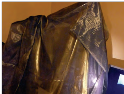
Figure 24 Transparent metallic cloth with a light shining directly onto it from the same angle it is viewed from is now reflective (metallic) and opaque
